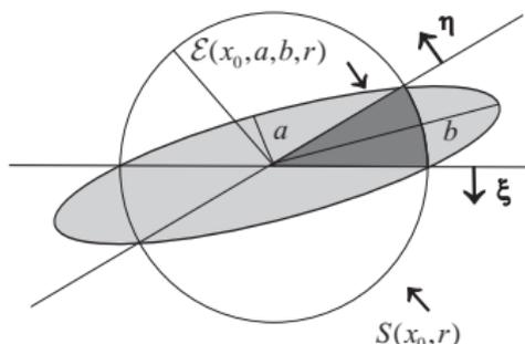
2d-ellipsoid contains the set  $W$  and has the minimum volume
